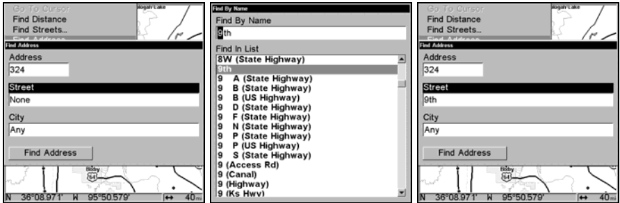
Find Address menu, left; Find Street menu, center, with Find By Name field active; street name entry complete, right.
