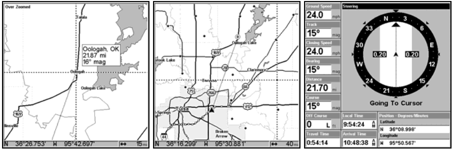
The 15-mile zoom figure at left clearly shows the dotted course line connecting your current position to your destination. The 40-mile zoom, center, shows both current position and destination on screen. The Navigation Page, right, will also show navigation information.
