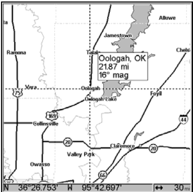
Navigate to cursor. In this example, the cursor has selected the town of Oologah, Oklahoma.
