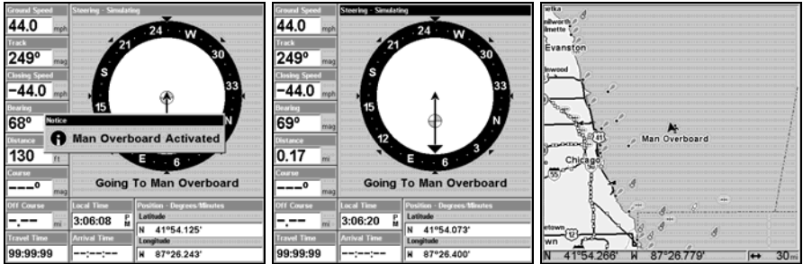
Navigating to Man Overboard: Man Overboard Activated message, left, Navigation Page, center, Map Page, right. The MOB is to the starboard of the vessel; the GPS shows which direction to steer for the rescue.
