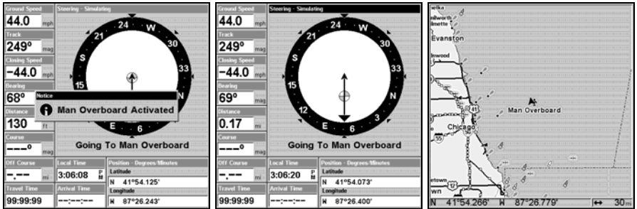
Navigating to Man Overboard: Man Overboard Activated message (left). Navigation Page, center, Map Page (right). The victim is to the starboard of the vessel. The GPS shows which direction to go for the rescue.
