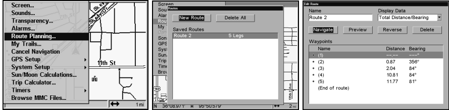
Route Planning command on Main Menu (left); Routes menu (center); Edit Route menu (right) with navigate command is selected.
