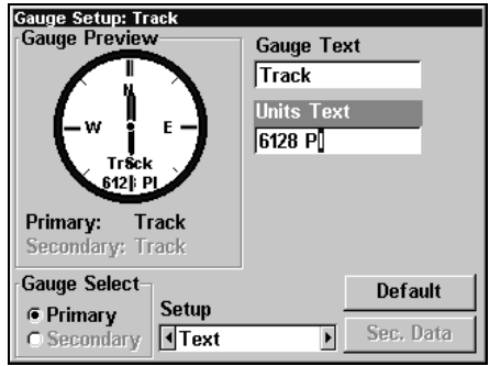
GlobalMap Text Setup menu (left) with transparent gauge labeled as "track"; Text Setup menu with destination house number entered in units text position (right).
