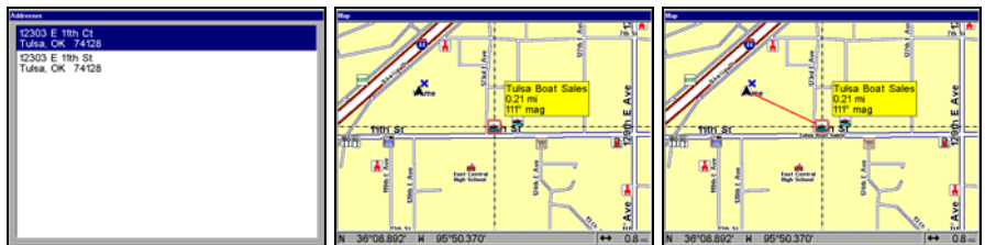
Address search result list (left). Map Page showing location of the address on the map, highlighted by cursor (center). After the address is located (right) you can navigate to it.
