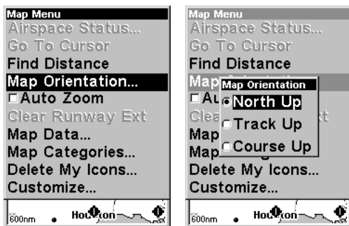
Map Menu, left, Map Orientation window with the North Up map orientation option selected.
