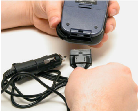
Attach external power cable to iFINDER.
