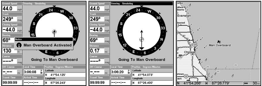
Navigating to Man Overboard: Man Overboard Activated message (left), Navigation Page (center); Map Page (right). The victim is to the starboard of the vessel. The GPS shows where to go for the rescue.
