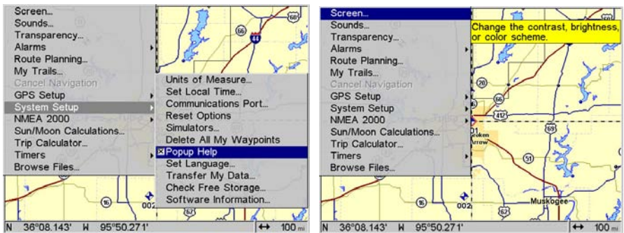
System Setup menu (left) with Pop-up Help command highlighted. The Pop-up Help message for the Screen command (right).
