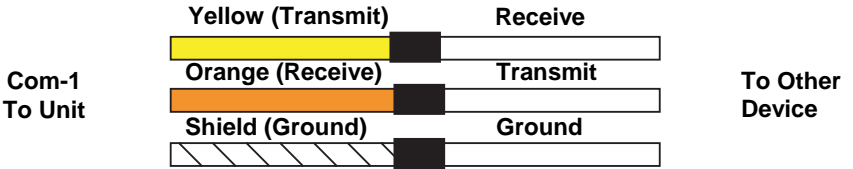
Com-1 wiring to exchange information with another device.
