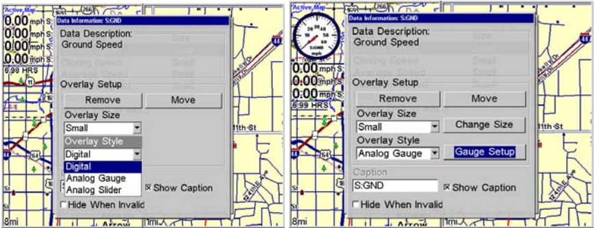
The GlobalMap Baja Data Information menu (left) with the Overlay style window activated. After choosing analog, the Analog Setup button appears (right).
