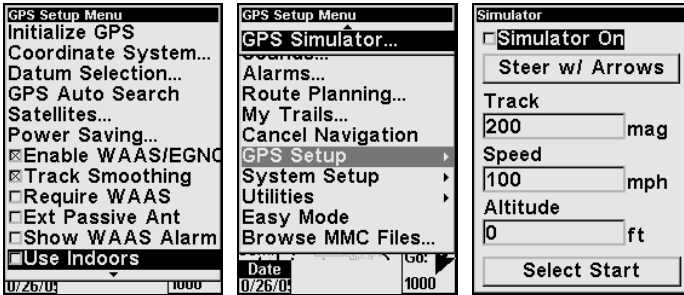
GPS Setup Menu with Use Indoors selected (left). Scroll past Use Indoors and GPS Simulator will appear at the top of the screen (center). The GPS Simulator menu (right).
