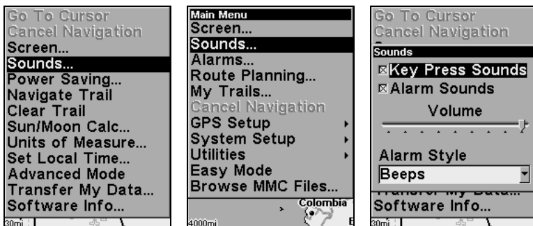
Sounds command: left, Easy Mode; center Advanced. At right, the Sounds menu.
