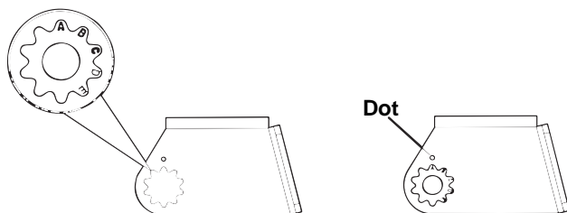
Align plastic ratchets in bracket.
