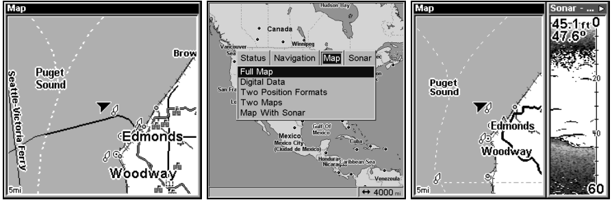
The full Map Page (left). Pages Menu with the Map option list (center). The Map with Sonar split screen (right).
