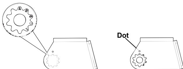
Align plastic ratchets in bracket.
