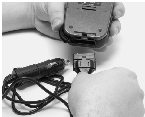
Attach external power cable to iFINDER.
