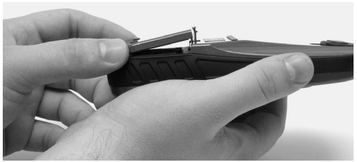
Remove iFINDER battery cover.
