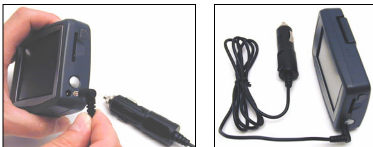
Attaching power cable to iWAY.
