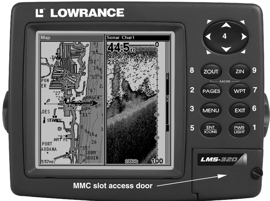
LMS-320 sonar/GPS unit, front view, showing map with sonar split screen, keyboard and access door for the MMC slot.
