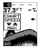
To stop the chart, first clear any menu from the screen by pressing the ON/ CLEAR key. You can't stop the chart while a menu is displayed. Now press the up arrow key. The chart will freeze and the word "STOP" appears at the top right portion of the screen. To start the chart, press the up arrow key again.
