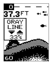
The level chosen by the X-25B when it's first turned on is usually adequate for most conditions. Experiment with your unit to find the Grayline setting that's best.
