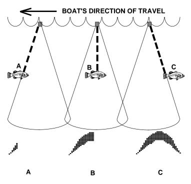
Large fish will arch, but turn the sensitivity up in deeper water to see the arch. Because of water conditions, such as heavy surface clutter, thermoclines, etc., the sensitivity sometimes cannot be increased enough to get fish arches.
