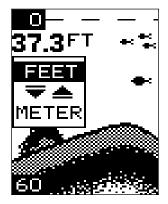
switch to metric, the up arrow to switch to feet. Displays show in feet when the unit is first turned on. The menu will clear automatically after a few seconds or you can press the ON/CLEAR key to clear the screen.
