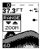
This is the zoom size menu. Zoom size is the distance between the upper limit and the lower limit. The upper limit shows at the top left corner of the screen. The lower limit is in the bottom left corner. For example, if the upper limit is 40 feet and the lower limit is 70 feet, the zoom window size is 30 feet. The word "TRACK" appears in this menu when you first activate the zoom as shown below. This means the X-25B is tracking the bottom in a zoom window, always keeping it on the display.
