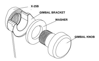
Attach the X-25B to the gimbal bracket using the supplied gimbal knobs and washers as shown above.
