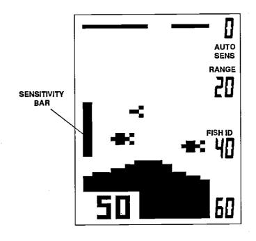
With high sensitivity settings, a second bottom echo (second echo) may appear. This is normal. It's caused by the returning signal reflecting off the surface of the water. Then it makes a second trip to the bottom and back again.
