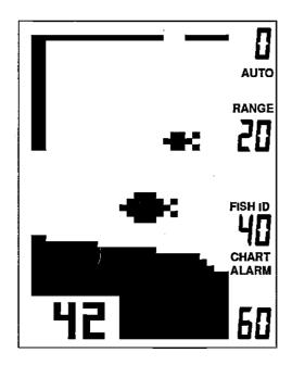
When the "Chart Alarm" signal is on, the alarm is active. If you wish to view the Chart Alarm bar, simply press the CHART ALARM key. The bar will be displayed for eight seconds. Any target that appears on the left side of the screen in the area covered by the chart alarm bar will trigger the alarm.
