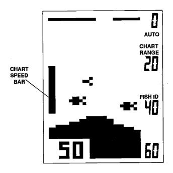
To view the chart speed without changing it, press the CHART SPEED key. The chart speed bar will appear for eight seconds.
