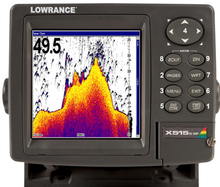
Sonar unit, front view, with keyboard. X-515cDF shown.
