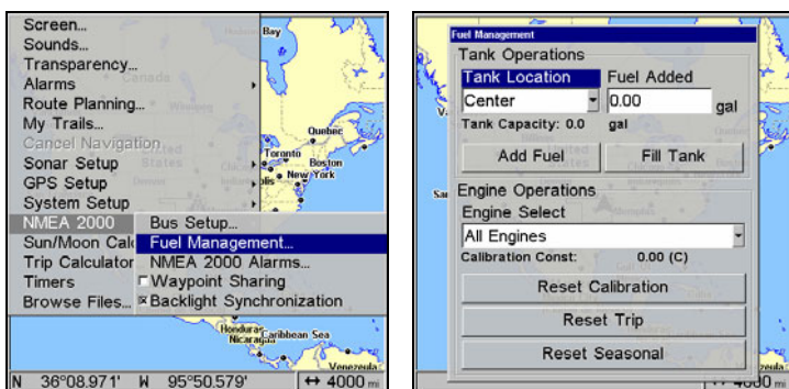
Fuel Management highlighted on the NMEA 2000 menu (left). Fuel Management menu (right).
