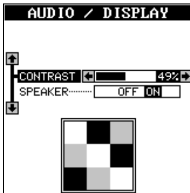
Audio/Display menu turns the sound off or on and adjusts screen contrast.
