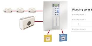
In the networked Extinguishing Control Panel LCnet216, up to 127 extinguishing systems with a total of 127 flooding zones can be implemented. Each extinguishing system can control up to 32 flooding zones, and each LCnet sectional control panel can administrate up to 8 flooding zones.
