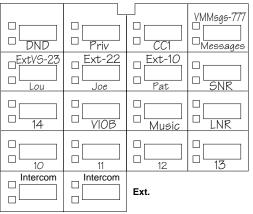
page 11.) The 34-button telephone has 15 lines assigned, and the Intercom Autodialer is programmed with Intercom Auto Dial and Manual Signaling buttons for 31 extensions; the order of extensions has been changed to begin with extension 11 on the top left button. The user's 18-button telephone has 5 individual lines assigned; the other 11 buttons are used for Intercom Auto Dialing and dial-code features.
