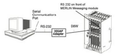
The MERLIN Messaging System supports one terminal session at a time. If a session is in effect through the Remote Maintenance Device (RMD) at the time the serial connection is being established, the MERLIN Messaging System ignores all input from the serial connection.
