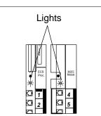
Check the green lights on the fronts of the modules. If a single light is out, power down the carrier, then power up the carrier. If both lights are out, power down the carrier, reseat both modules, then power up the carrier. If the lights are still out, in the Continental U.S., call the hotline at 1-800-721-7071. Outside the Continental U.S., contact your Lucent Technologies Representative or local Authorized Dealer.
