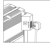
Press the power cord firmly into the power jack on the carrier. Plug the other end of the power cord into a properly grounded three-prong wall outlet not controlled by a switch.
