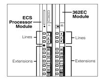
A) Label the lines and extension jacks. B) Connect the line and telephone cords to the appropriate jacks on the new module. C) Route each cord through the hook on the front of its module. D) Connect the free end of each phone cord to the modular wall jacks for system extensions.
