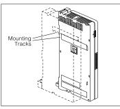
A) Slide the second module off the PARTNER Endeavor processor module and put it aside. B) Slide the 362EC module onto the PARTNER Endeavor processor module, making sure the mounting tracks interlock, as shown in the side view.
