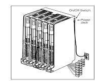
A) Plug the power cord into a properly grounded three-prong wall outlet not controlled by a switch.
