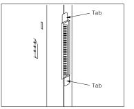
Before installing any modules, make sure the clear, plastic protector has been removed from the connector area on the rear of each module. To remove the protector, grasp the tabs on the ends of the protector and lift.
