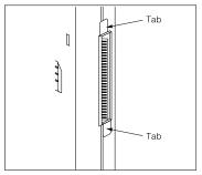
Remove the clear, plastic protector from the connector on the right side of the new 362EC module by grasping the tabs on the ends of the protector and lifting. If you are upgrading from a stand-alone system, also remove the protector from the wall-mounted PARTNER Endeavor processor module.
