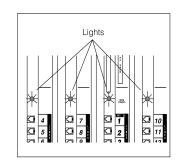
Check the green lights on the fronts of the modules. If a single light is out, power down the carrier, then power up the carrier. If multiple lights are out, power down the carrier, reseat both modules, then power up the carrier. If the lights are still out, in the Continental U.S., call the hotline at 1-800-721-7071. Outside the Continental U.S., contact your Lucent Technologies Representative or local Authorized Dealer.
