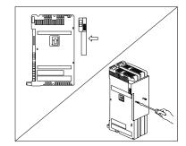
Attach the 2-Slot carrier to the top right side of the two modules:
