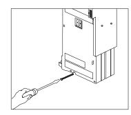
Insert the 3 1/2" #8 screw into the bottom of the modules. Tighten it until the mounting tracks of the PARTNER Endeavor processor module are flush against the wall with a 3/8" (1 cm.) gap between the wall and the rest of the PARTNER Endeavor processor module. Do not overtighten, the modules will warp.
