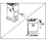
3 If you are replacing the second module in a two-slot carrier, remove the two #4 screws holding the carrier in place and gently pull the carrier off the modules.
