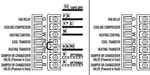
\* If both "Y" and "C" wire are present, tape off "C" wire.
