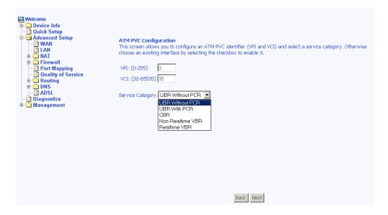
The ATM PVC Configuration screen allows you to configure an ATM PVC identifier (VPI and VCI) and select a service category.
