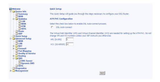
Following is the Connection Type screen where you select the type of network protocol and encapsulation mode over the ATM PVC that your ISP has instructed you to use. The following is a PPPoA example. Click on **Next** to continue.
