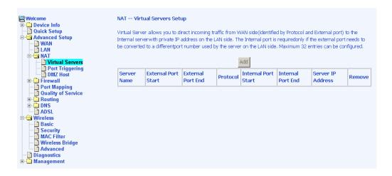
In the next screen, select the virtual server from the drop-down list and complete the server IP address, then click on the **Save / Apply** button.
