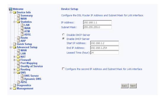
If you have a second IP address and subnet mask for the LAN interface, click on the checkbox to configure it. See below example below.
