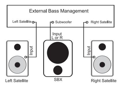
In this setup, you will want to set the Subwoofer LPF control knob to the desired cutoff frequency for the SBX. Once again, the Satellites HPF control knob is not operational with the HPF Bypass switch set to "On."
