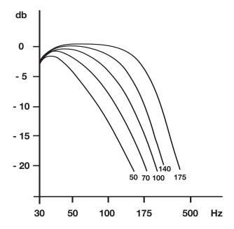
This crossover network consists of two main components: a 2nd order (12 db/octave) low-pass filter that limits the upper frequencies that the subwoofer has to reproduce (shown above), and a high-pass filter that limits the lower frequencies the satellite monitors have to reproduce (shown below). The Subwoofer LPF cutoff frequency (#4) and Satellite HPF cutoff frequency (#5) controls adjust frequencies of the low- and high-pass filters, respectively. Both have a range of 50 to 180 Hz.
