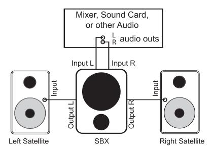
Once you have completed this setup, you must set the Subwoofer LPF control knob and the Satellites HPF control knob for your particular needs. Please see the section, "Optimizing the Rear Panel Settings" for information on how to do this. Also note that the HPF Bypass switch is set to "Off" in this scenario.
