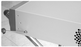
Dismantle the top cover, open the cabinet
