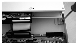
Dismantle the HD bracket
