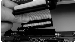
Connect HD data line to IDE port
