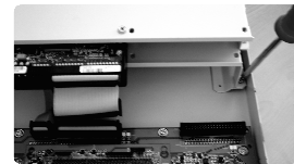
Connect the HD bracket
