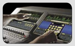
major features and functions at your fingertips as "virtual" controls, with big, button-style graphics and a bare minimum of hierarchy. With advanced 5-wire technology and a proprietary tracking algorithm, the touch screens deliver incredibly accurate response. And they're built tough too, with an operating life that's rated at over 35 million finger pokes.
