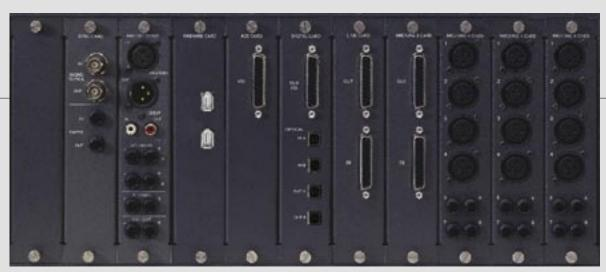
The Digital X Bus' full rear-panel card cage allows you to configure I/O exactly as you see fit, with analog mic /line cards, digital cards, FireWire cards and more. It comes with the Sync Card and Mix Out Card pre-installed.
