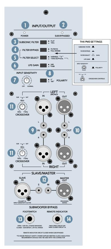
Frequencies below the crossover frequency are sent to the subwoofer, and frequencies above the crossover frequency are sent to the LEFT and RIGHT OUTputs, which are connected to the main/satellite speakers.
