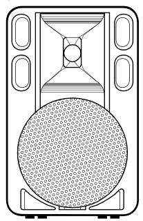
The ART500 is a full-range two-way professional passive speaker system that combines high power, wide bandwidth, and the reduced weight of a special hybrid construction for fixed-installation systems. The 15" low-frequency transducer, in combination with a 2" titanium compression driver coupled to an integral  $80^{\circ} \times 60^{\circ}$  constant directivity polynomial horn, form an extremely powerful package for any small to medium-sized sound reinforcement application.
