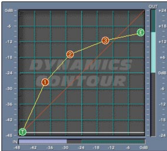
Expansion and compression together to "level" a signal
