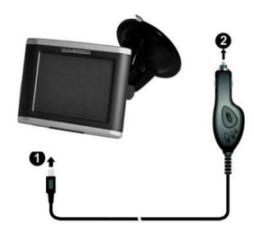
To connect the charger, insert the terminal (1) into the connector on the navigator and terminal (2) into the car's cigar lighter socket.
