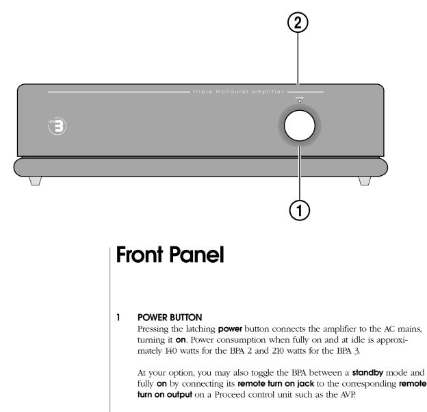
When first powered up, the BPA will always go to fully **on**, regardless of the signal present at its **remote turn-on jack**. If the control unit then turns on, the amplifier will remain on; thereafter, the two will remain in sync. If power is removed from the BPA, it will automatically re-sync with the control unit in the course of normal operation. No user intervention is required, beyond simply turning the system on and off from the control unit.
