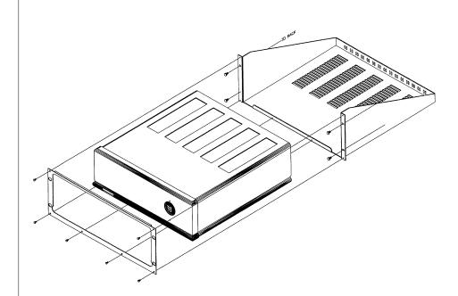
The mounted amplifier and rack mount kit occupies 5 standard rack units of height.
