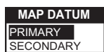
Figure D. Be sure the map datum matches the datum required for the maps or charts you are using.
