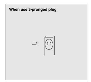
When use grounding adaptor, make sure the receptacle box is fully grounded.
