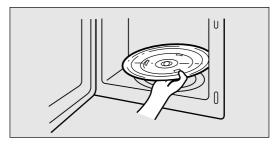
The roller guide and oven cavity floor should be cleaned regularly to avoid excessive noise.
