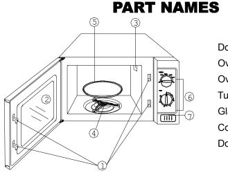
Door Safety Lock System Oven Window Oven Air Vent Turntable roller Glass Tray Control Panel Door Release Button
