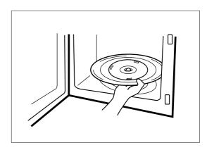
The roller guide and oven cavity floor should be cleaned regularly to avoid excessive noise. Simply wipe the bottom surface of the oven with mild detergent water or window cleaner and dry. The roller guide may be washed in mild sudsy water.
