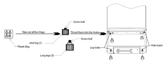
Note : Must screw the short leg into the base bracket!
