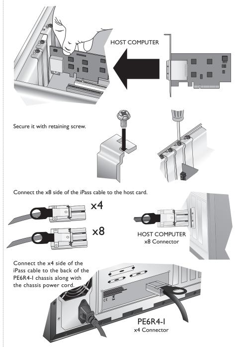
Repeat the process for all other PCI or PCI-X peripherals you wish to install in the chassis.
