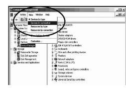
Open "ACPI (BIOS)" > Open "PCI Bus" > Click the "+" sign several times until you reach a PCI Express Root Port with a PCI Standard PCI-to-PCI Bridge beneath it.
