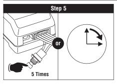
To exit programming push the switch on/off 5 times or wait 15 seconds and the system will automatically exit the "Automatic Code Learning" mode.
