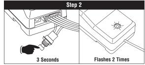
Press and hold the button on the receiver for **3** seconds. The LED on the receiver will flash 2 times and then turn off. Release the switch. You are now in "Automatic Code Learning" mode.
