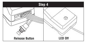
Release the receiver's button and the LED will turn off. Repeat Steps 2-4 to program additional remotes. **Note:** Up to 4 remotes can be programmed.
