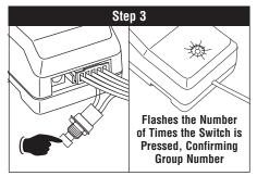
Press the switch on/off the number of times according to the radio manufacturer's **Group** number listed in the Manufacturer's Code Look-Up Table.
