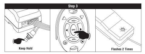
While still pressing the button on the receiver, press and release the SRC button on the remote until the LED on the receiver flashes 2 times, indicating the code is learned.
