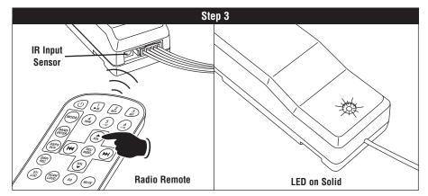
Within 15 seconds, aim the radio remote at the IR input sensor and push the "VOLUME UP" button on the radio remote.
