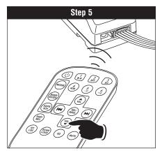
Repeat Step 3 and 4 for the remaining 7 buttons. Each button has a unique LED flash indicator confirming when they have been programmed.
