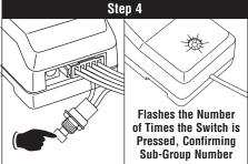
Press the switch on/off the number of times according to the radio manufacturer's **Sub-Group** number listed in the Manufacturer's Code Look-Up Table.
