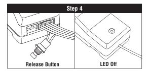
Release the receiver's button and the LED will turn off.
