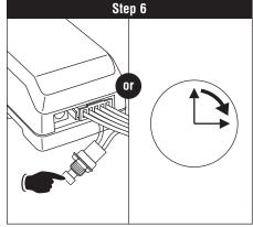
To exit programming push the switch on/off 3 times or wait 15 seconds and the system will automatically exit the "Manual Code Learning" mode.
