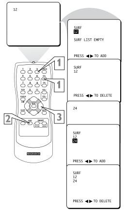
Press SURF repeatedly during TV viewing to scan through the channels in the SURF list.
