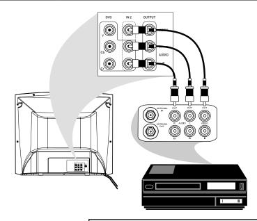
There are AUDIO and VIDEO IN 1 jacks at the lower-right corner of the rear of the TV. To view material playing on equipment connected here, press TV/AV/EXIT so VIDEO 1 is on the TV.
