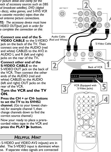
he S(uper)-Video connection on the rear of the TV can provide you with better picture detail and clarity for the playback of accessory sources such as DBS (digital broadcast satellite), DVD (digital video discs), video games, and S-VHS VCR (video cassette recorder) tapes than the normal antenna picture connections.
