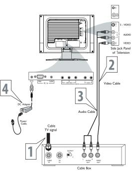
The AUDIO and VIDEO In jacks on the rear of the LCD TV enable quick connections of other equipment. Connect a VCR, DVD Player, Video Game, Camcorder, etc., to these jacks. To view the material playing on the other equipment, set the LCD TV to its AV Mode.
