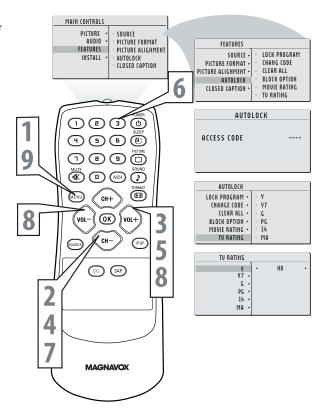
You can change the picture format size to match the type of program you are watching. Select the normal 4:3, EXPAND 4:3, or COMPRESS 16:9, or HD 4:3 aspect ratios.
