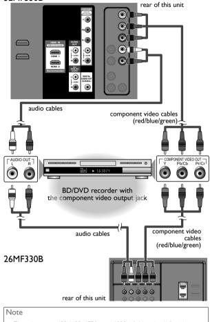
The unit accepts 480i/480p/720p and 1080i of video signals for this connection.
