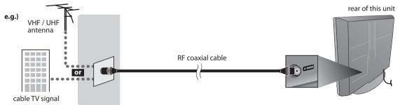
\* Once connections are completed, turn on the unit and begin initial setup. Channel scanning is necessary for the unit to memorize all available channels in your area. Refer to "Initial Setup" on page 17.
