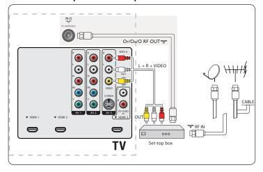
If your device has an S-VHS video jack: For improved picture quality, connect a S-Video cable with the S-Video input of AV3/side AV and connect the audio cables to the audio L and R input jacks of AV3/side AV.
