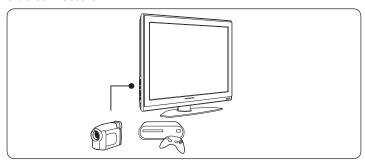
Use the TV side connectors to connect to mobile devices such as a high definition game console. You can also connect a pair of headphones.
