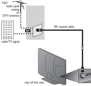
Once connections are completed, turn on the unit and begin initial setup. Channel scanning is necessary for the unit to memorize all available channels in your area. [Initial Setup] IIII p.15
