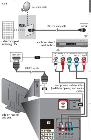
You can also connect this unit to the cable receiver or satellite box other than the HDMI or the component video output jacks because they might have different output jacks.
